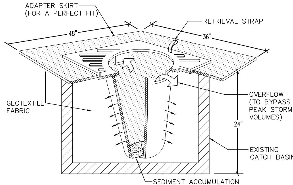
PROVIDE CATCH BASIN SEDIMENT PROTECTION WITH STREAMGUARD BASIN INSERT #3003, FROM FOSS ENVIRONMENTAL OR APPROVED EQUAL
