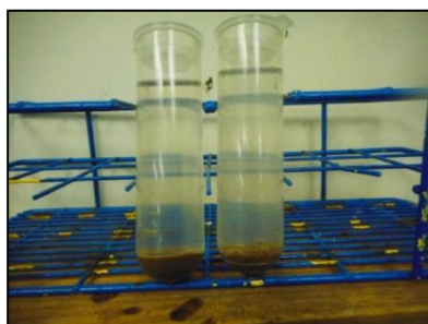
Photo 5: Left Spun Without Polymer Right Spun With Polymer
