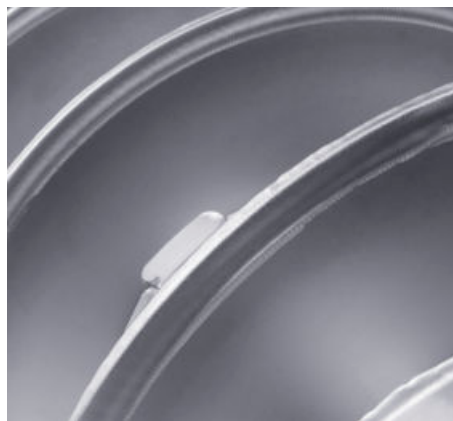
Figure 6. Flame sprayed tungsten carbide wear protection on conveyor flights
