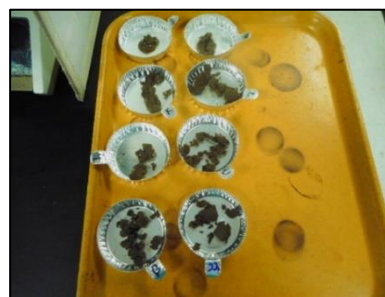
Photo 6: Spin Dewatered Cakes 5, 10, 15, 20 Minute Spins at 3000g's
