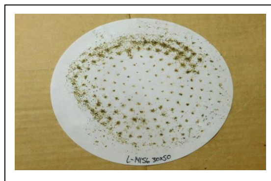
Photo #2: 30X50 Mesh Fraction
